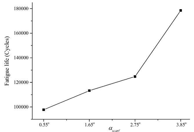
Fig. 17. Fatigue life versus the scarf angle.
