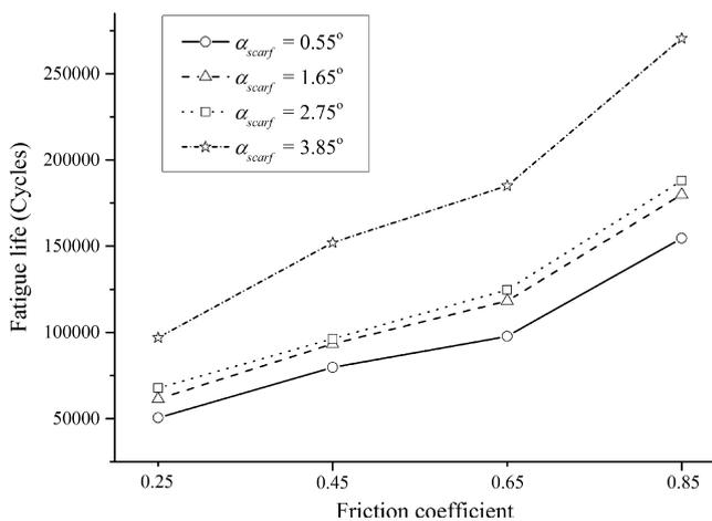
Fig. 35. Fatigue lives versus the friction coefficient and scarf angle.
