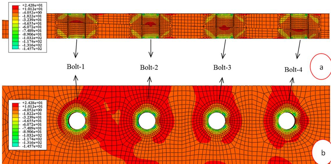
Fig. 9. Distribution of the longitudinal stress (MPa): (a) along the depth direction on the area around the bolt hole and (b) on the surface of the plate.
