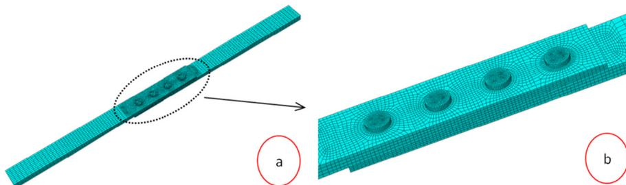
Fig. 8. The established finite element model: (a) the global view and (b) the local view.
