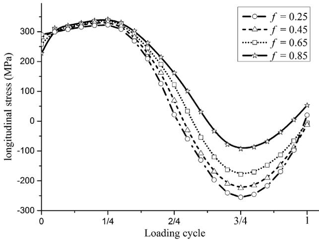
Fig. 22. Change of the longitudinal stresses (MPa) within one loading cycle with respect to different friction coefficients.
