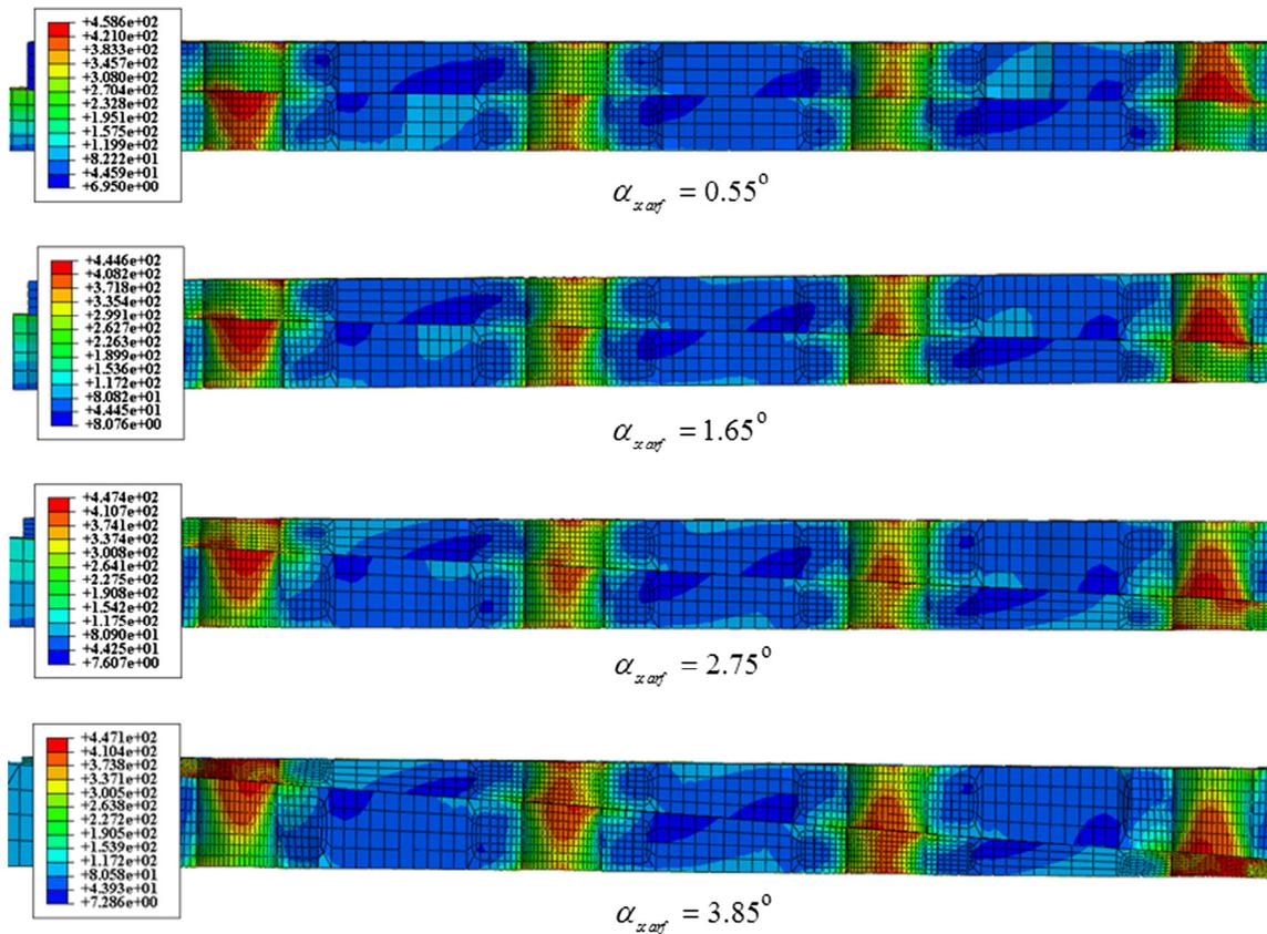
Fig. 14. Distribution of the von Mises stress (MPa) with respect to different scarf angles.
