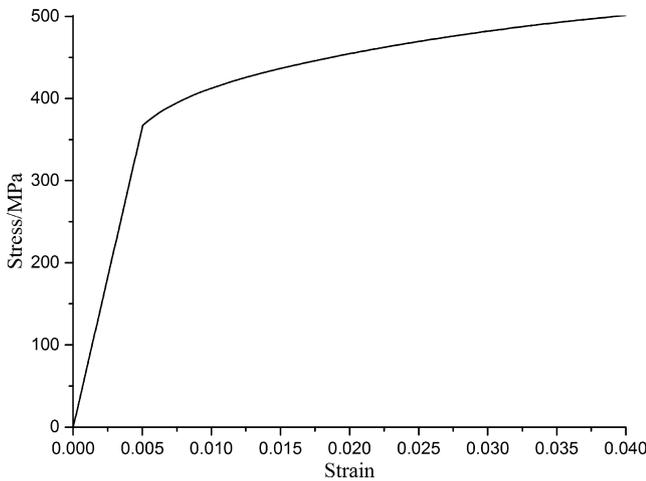
Fig. 1. Stress-strain curve for the 2024-T351 aluminium alloy.
