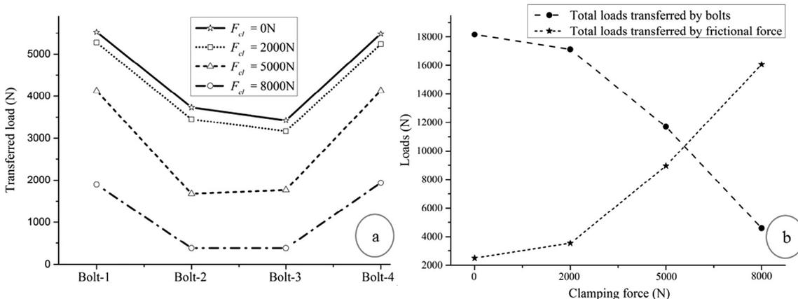
Fig. 30. (a) Effect of the clamping force on load transferred by each bolt and (b) total loads transferred by the bolts and by the frictional force.
