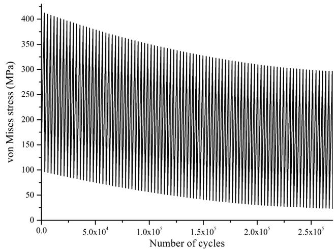
Fig. 12. The evolution curve of the von Mises stress at the critical element versus the number of cycles.
