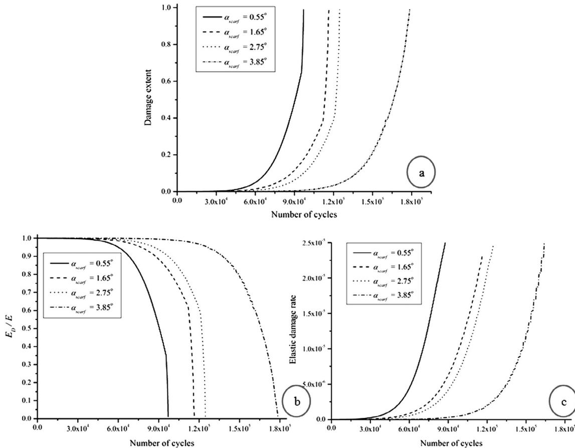
Fig. 18. (a) Damage extent versus the number of cycles with respect to different scarf angles, (b) reduction in the equivalent Young's modulus of the critical element and (c) the evolution curve of the elastic damage rate.
