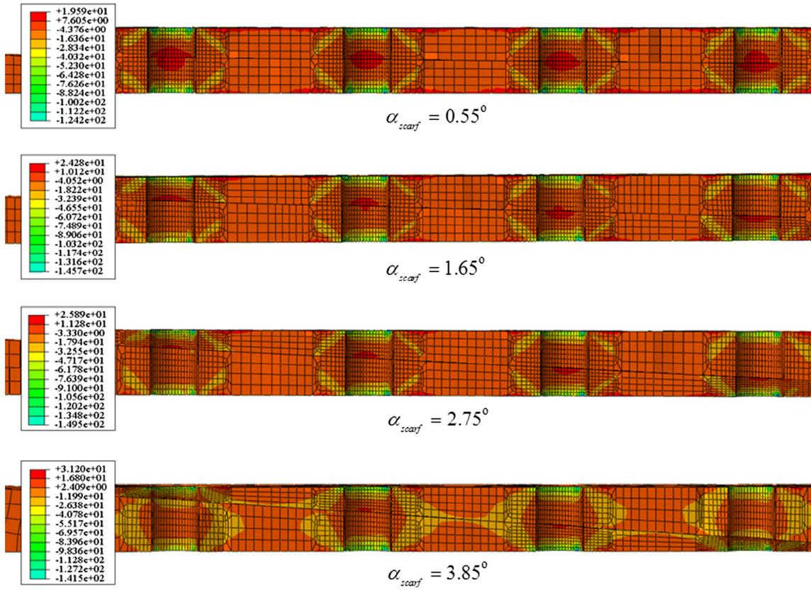
Fig. 13. Distribution of the longitudinal stress (MPa) with respect to different scarf angles.
