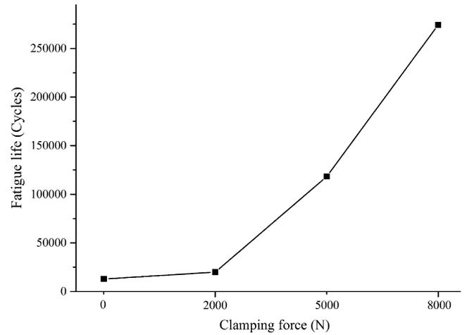
Fig. 31. Fatigue life versus the clamping force.
