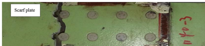
Fig. 5. Fracture photograph of the scarf plate.
