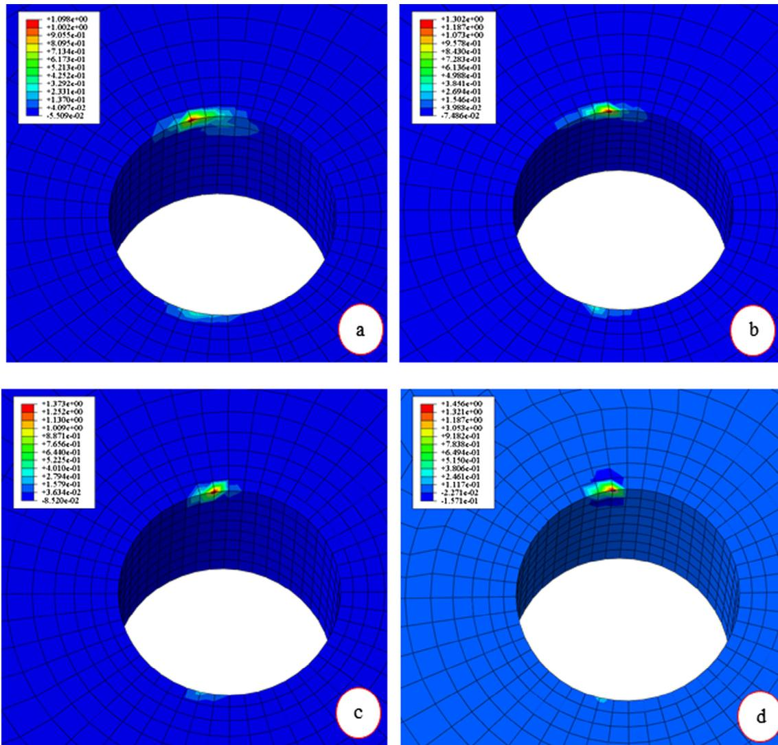
**Fig. 19.** Failure locations of the critical element corresponding to the different scarf angles (a) scarf angle = 0.55°, (b) scarf angle = 1.65°, (c) scarf angle = 2.75° and (d) scarf angle = 3.85°.
