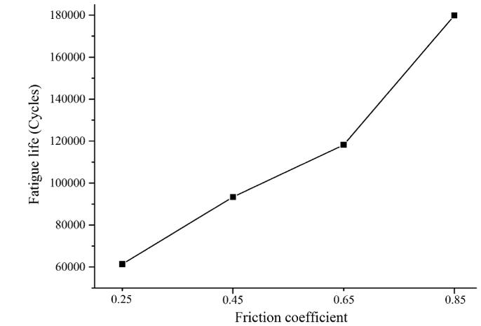
Fig. 24. Fatigue life versus the friction coefficient.
