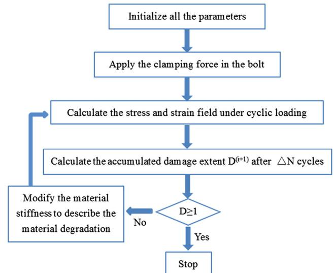
Fig. 6. The flowchart of the numerical calculation.
