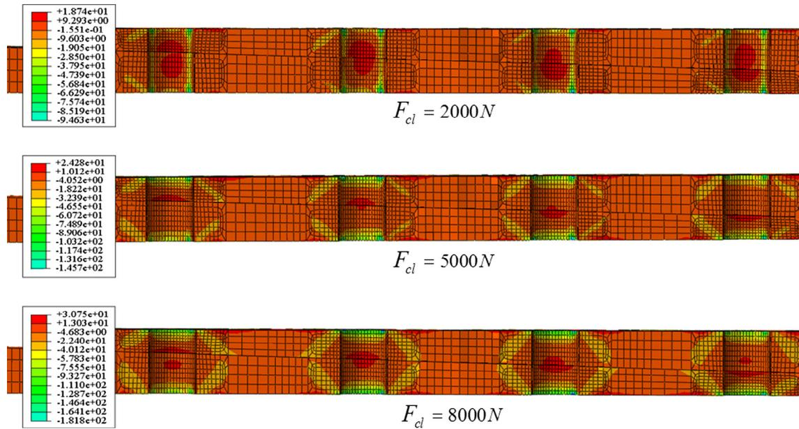
Fig. 27. Distribution of the longitudinal stress (MPa) with respect to different clamping forces.
