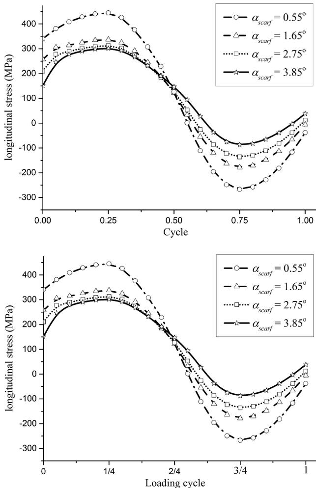
Fig. 15. Change in the longitudinal stresses (MPa) within one loading cycle with respect to different scarf angles.
