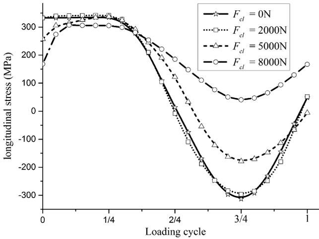
Fig. 29. Change in the longitudinal stresses (MPa) within one loading cycle with respect to different clamping forces.
