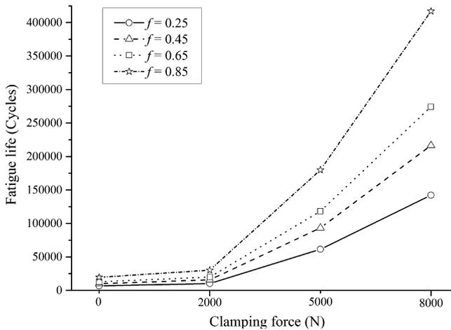
Fig. 33. Fatigue lives versus the clamping force and the friction coefficient.
