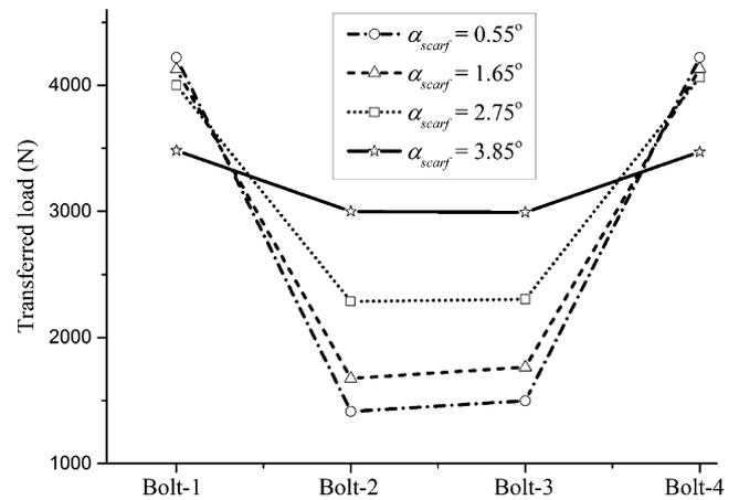
Fig. 16. Effect of the scarf angle on the load transferred by each bolt.
