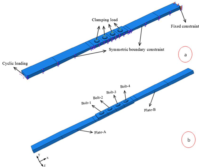
Fig. 7. One half of the model: (a) loads and constraint conditions and (b) schematic diagram of coordinate system and part name.
