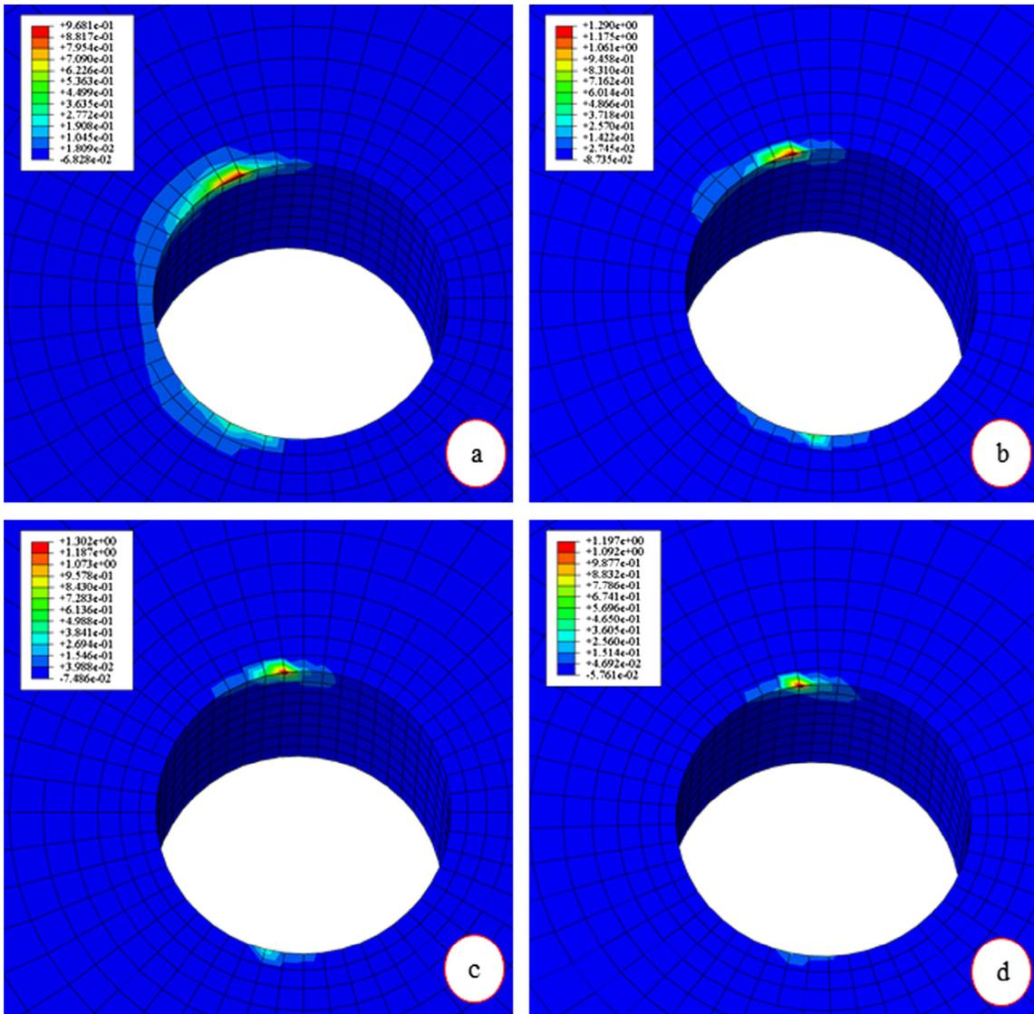
Fig. 26. Failure locations of the critical element corresponding to the different friction coefficient (a)  $f = 0.25$ , (b)  $f = 0.45$ , (c)  $f = 0.65$  and (d)  $f = 0.85$ .
