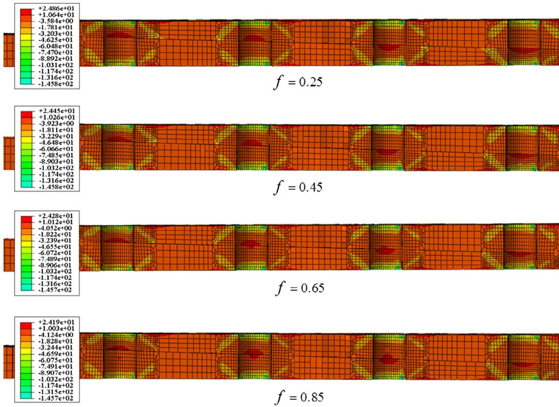
Fig. 20. Distribution of the longitudinal stress (MPa) with respect to different friction coefficients.
