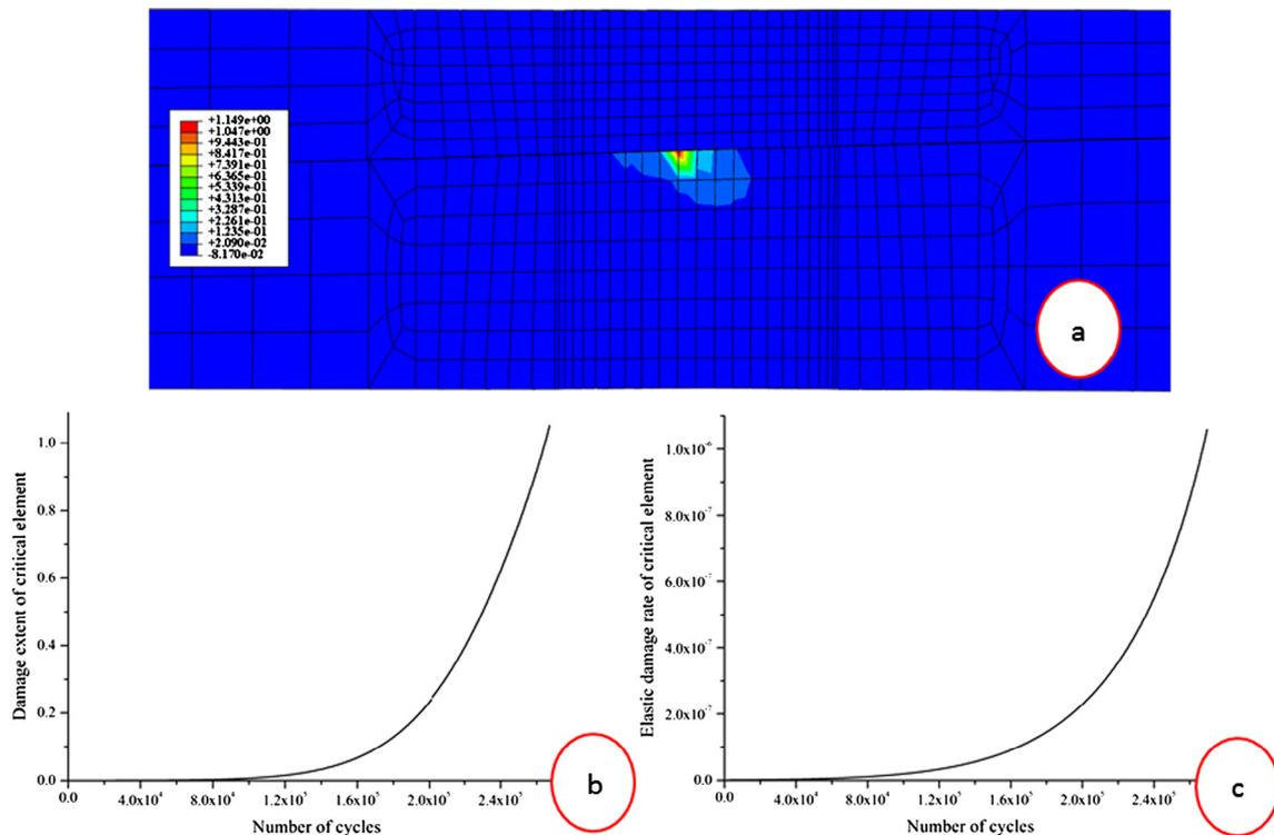
Fig. 11. Fatigue damage analysis: (a) damage field distribution of the local area, (b) the damage extent versus the number of cycles for the critical element and (c) the evolution curve of the elastic damage rate.
