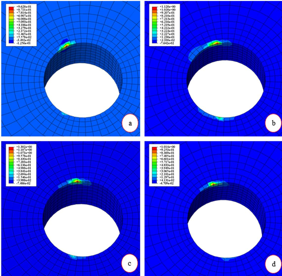
Fig. 32. Failure locations of the critical element corresponding to the different clamping force (a)  $F_{cl} = 0$ , (b)  $F_{cl} = 2000$ , (c)  $F_{cl} = 5000$  and (d)  $F_{cl} = 8000$ .
