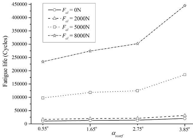
Fig. 34. Fatigue lives versus the scarf angle and the clamping force.
