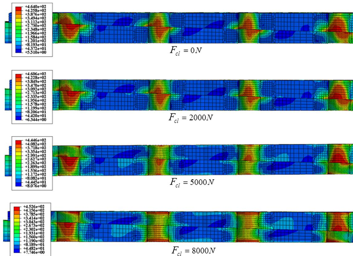
Fig. 28. Distribution of the von Mises stress (MPa) with respect to different clamping forces.
