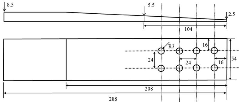
**Fig. 3.** Geometry of the scarf plate.
