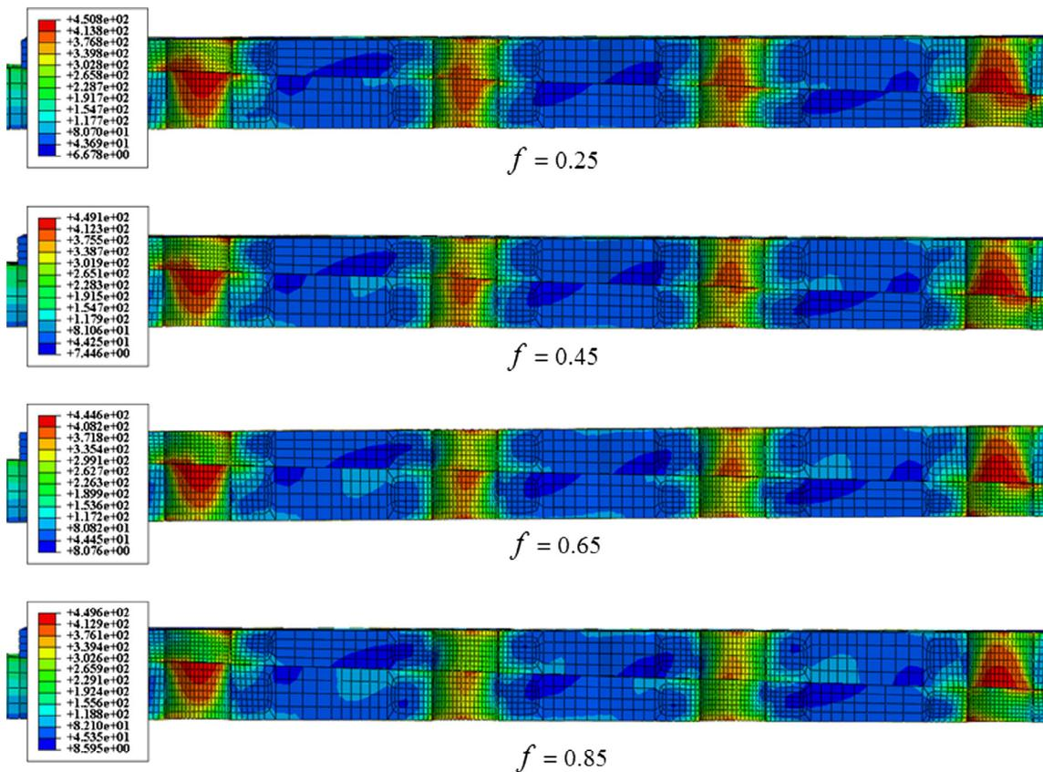
Fig. 21. Distribution of the von Mises stress (MPa) with respect to different friction coefficients.
