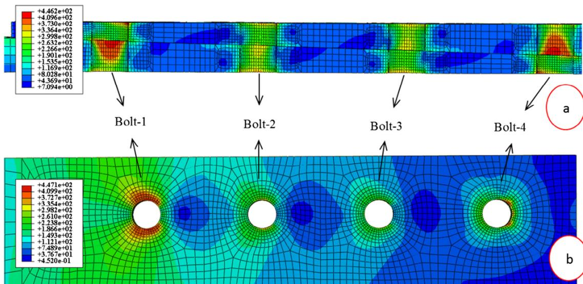
Fig. 10. Distribution of the von Mises stress (MPa): (a) along the depth direction on the area around the bolt hole and (b) on the contact surface of the scarf plates.
