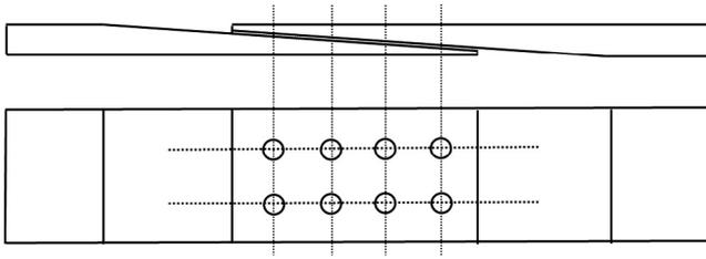
Fig. 4. Schematic diagram of the assembly of the scarf bolted joints.
