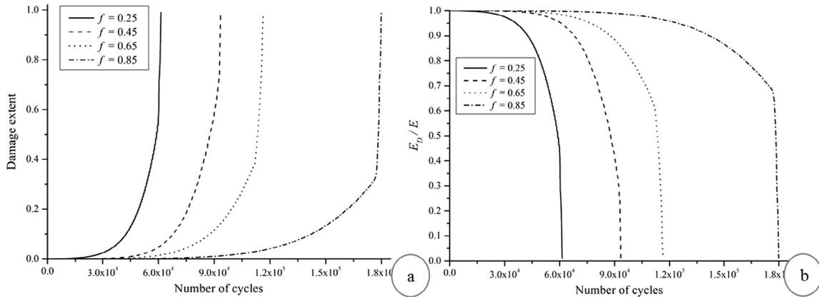
Fig. 25. (a) Damage extent versus the number of cycles with respect to different friction coefficients and (b) reduction in the equivalent Young's modulus at the critical element.
