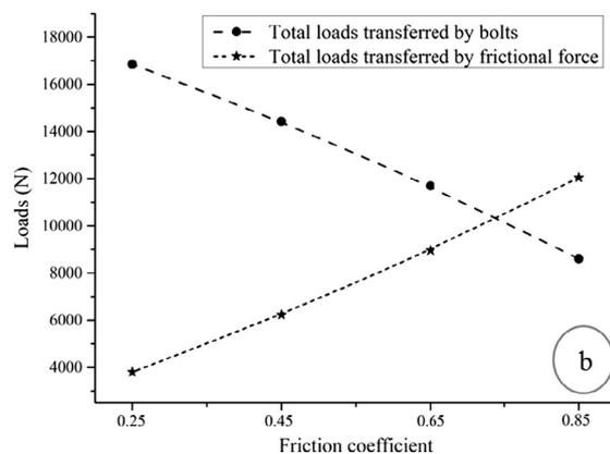
Fig. 23. (a) Effect of the friction coefficient on the load transferred by each bolt and (b) total loads transferred by the bolts and by frictional force.
